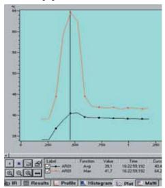
The time trend analysis of the maximum and average temperatures of a faulty component, using the specially developed machine vision software.
